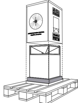
After removing the strapping securing the box to the pallet, remove the screws at the bottom of the box, lift and remove the lid like in the image.
