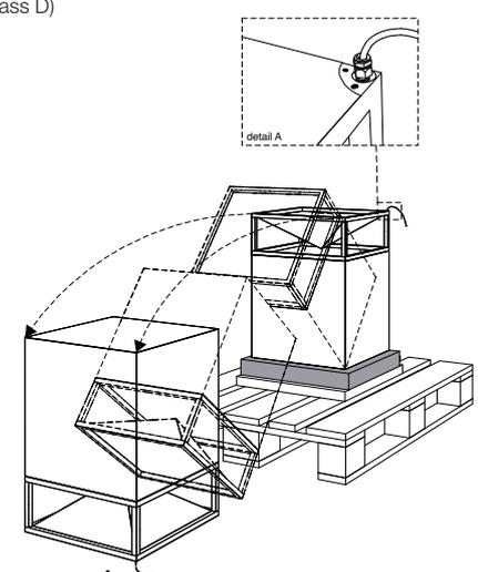
While turning the module, pay particular attention not to squeeze and damage the conduit and the cable sticking out below the base; the conduit must be accommodated in a special slot in the ground.
