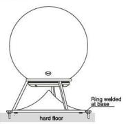
In the case of installations on hard floors, like stone or wood, AS provides a suitable anti-theft base as an accessory, which has 3 rings welded on its border, to secure it on the floor using the screws considered more appropriate by the installer according to the typology of the floor.
