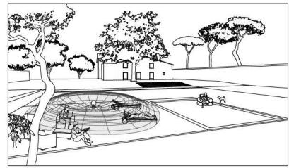
Installation precautions: When installing the Sphere outdoor in presence of an irrigation system make sure water DO NOT directly reach the speaker below, either from the bass reflex hole or bouncing on the deflector.
