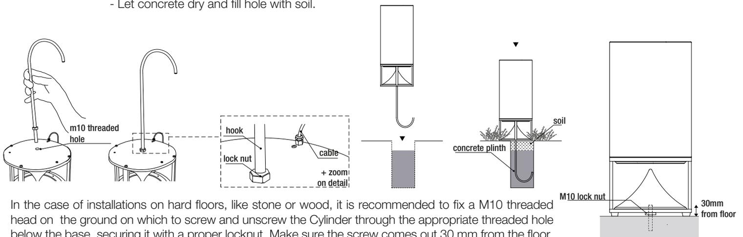
In the case of installations on hard floors, like stone or wood, it is recommended to fix a M10 threaded head on the ground on which to screw and unscrew the Cylinder through the appropriate threaded hole below the base, securing it with a proper locknut. Make sure the screw comes out 30 mm from the floor.
