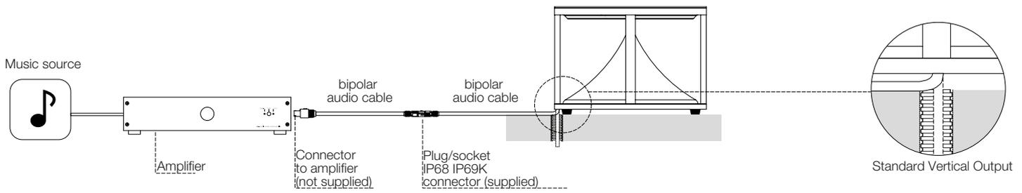
**Lighting Mood Output (optional):** the Lighting Mood bases have two cables coming out from below, the acoustic and the electrical one; refer to the following scheme for installation:
